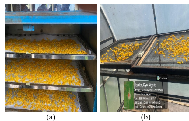
Figure 3. Interior views of the dryers showing thinly spread sliced mango chips a: NSPRI multi-crop dryer; b: NSPRI PSSD
